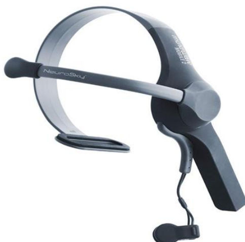
Рис. 3. Нейрогарнитура NeuroSky MindWave Mobile 2 Fig. 3. NeuroSky MindWave Mobile 2 Neural Headset
